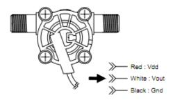
3.0 Mounting method Horizontal mounting, maximum 30 degree lifting.
